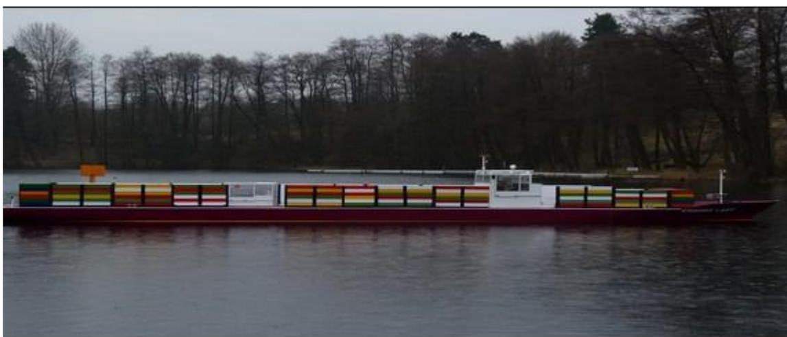
Model of a VLCS with the bridge located at the bow
