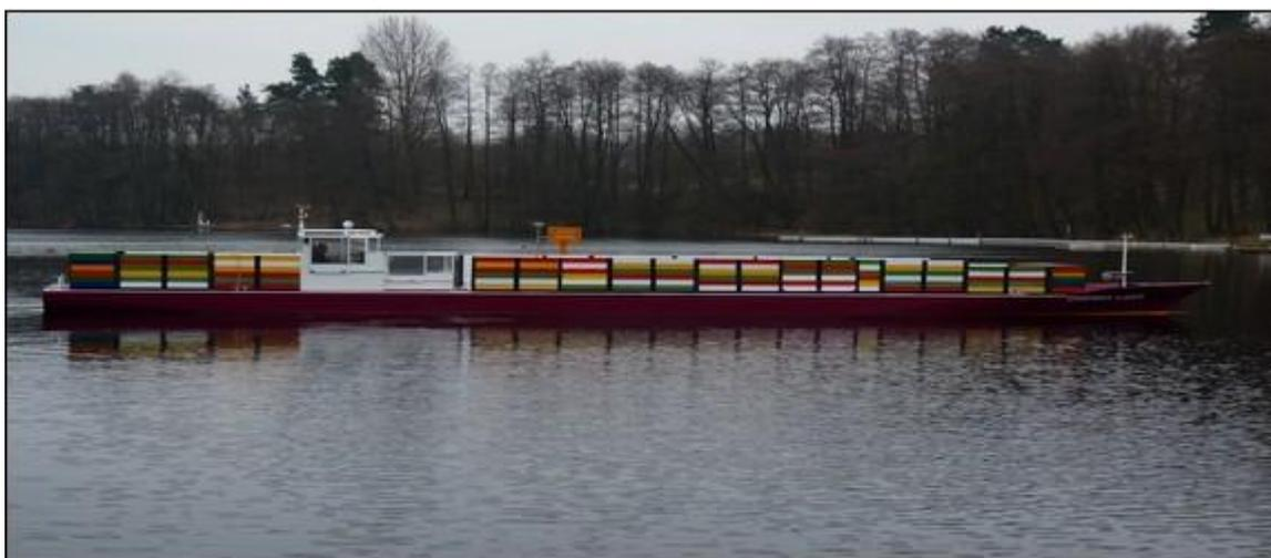
Model of a VLCS with the bridge located at the stern
