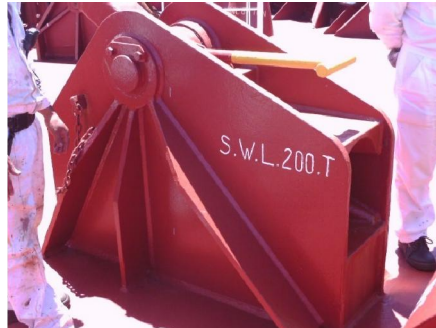
Figura 16: Chain Stopper de proa – 200 TON
