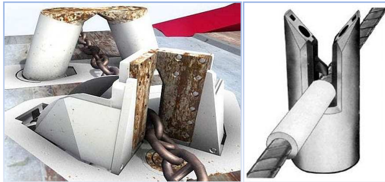
Figura 44 Shark Jaw (esq.) e Karm Fork (dir.)
