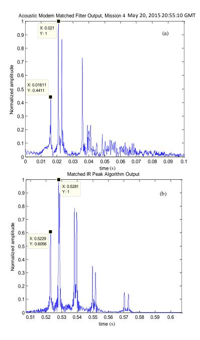
Figure 22. Acoustic Modem (a) Matched Filter Output and (b) Matched Peak IR Algorithm Output.
