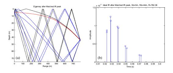
Figure 23. (a) Eigenrays and (b) Ideal IR after Matched Peak IR Processing.
