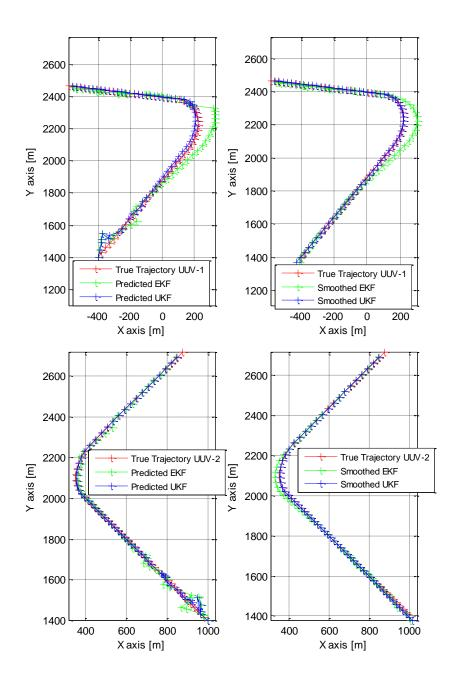
Figure 46. Tracking Results, Measurement Failure Case Plus Noise
