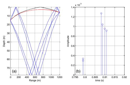
In ray tracing, eigenrays are defined as rays that connect the source to a particular receiver location. Note that, in this example, the first group of arrivals has smaller amplitude than the second group.
