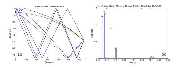
Figure 29. (a) Eigenrays and (b) Ideal IR after Matched Peak IR Processing.
