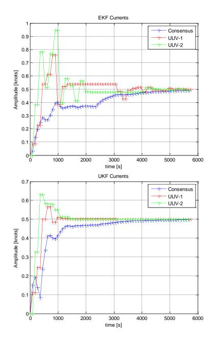
Figure 45. Consensus Current, Measurement Failure Case
