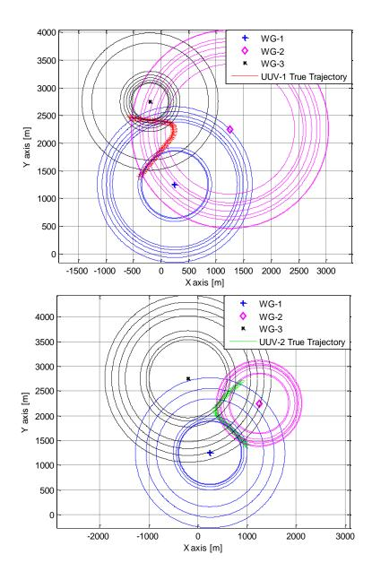
Figure 42. Distance Measurements in xy-Plane, Measurement Failure Case
