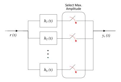
Figure 6. Multi-hypothesis Detector or "Bank" of Matched Filters
