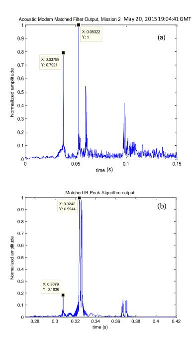
Figure 25. Acoustic Modem (a) Matched Filter Output and (b) Matched Peak IR Algorithm Output.
