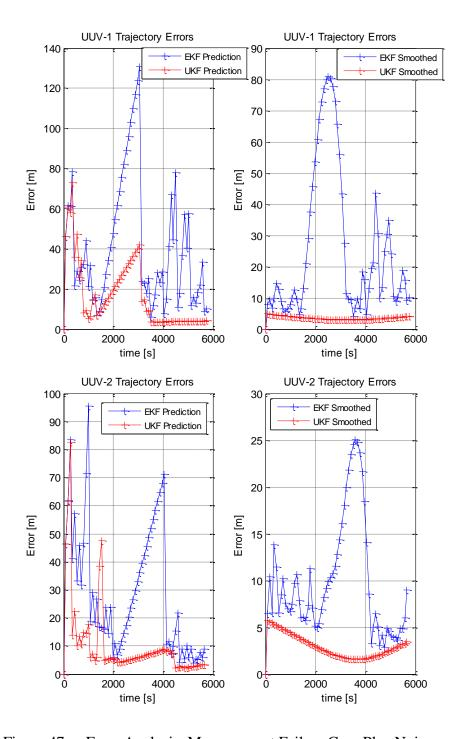
Figure 47. Error Analysis, Measurement Failure Case Plus Noise
