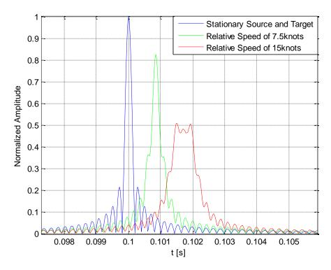
The characteristics of the LFM pulse are: T=50ms, B=5 kHz sweeping from 9 kHz to 14 kHz (TB=250).
