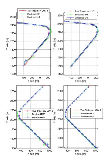
Figure 43. Tracking Results, Measurement Failure Case
