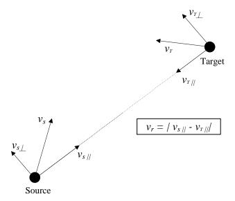
Figure 5. Relative Radial Speed between Source and Target
