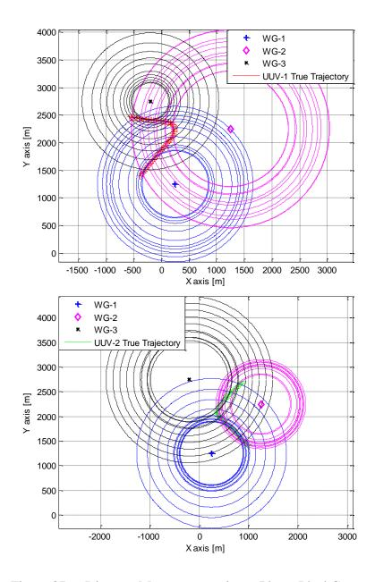
Figure 37. Distance Measurements in xy-Plane, Ideal Case
