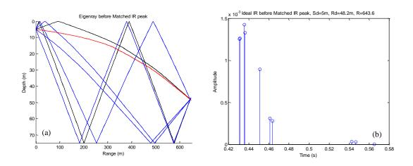
Figure 27. (a) Eigenrays and (b) Ideal IR before Matched Peak IR Processing.
