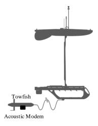
Figure 55. Wave Glider Equipped with Towfish Modem. Adapted from Liquid Robotics, <a href="https://www.liquid-robotics.com/">https://www.liquid-robotics.com/</a>
