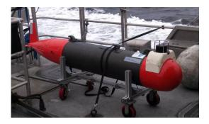
Figure 53. Coastal Glider Rigged with Syntactic Foam Mount for Acoustic Modem
