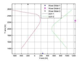
Figure 49. True Trajectory of UUVs (Experiencing Different Currents)
