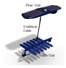
Figure 54. Liquid Robotics Wave Glider Model SV2. Source: Liquid Robotics, <a href="https://www.liquid-robotics.com/">https://www.liquid-robotics.com/</a>
