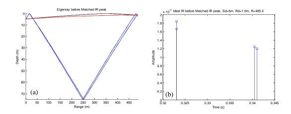
Figure 24. (a) Eigenrays and (b) Ideal IR before Matched Peak IR Processing.
