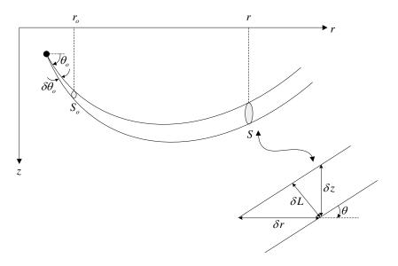
Figure 16. Geometry of a Ray Tube
