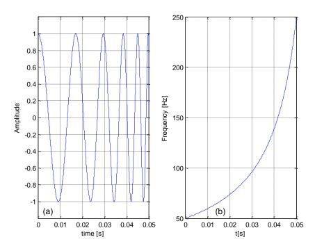
This HFM pulse is defined in the interval 0 < t < 50ms with B = 200Hz (TB = 10).
