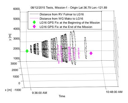
Figure 59. Mission-1, Time Evolution of the Distance Measurements
