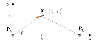
Figure 81. UUV and Two Reference Points
