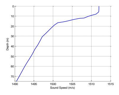
Figure 12. Sound Speed Profile Measured in Monterey Bay on August 12, 2015
