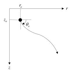
Figure 15. Rays 2D Initial Conditions
