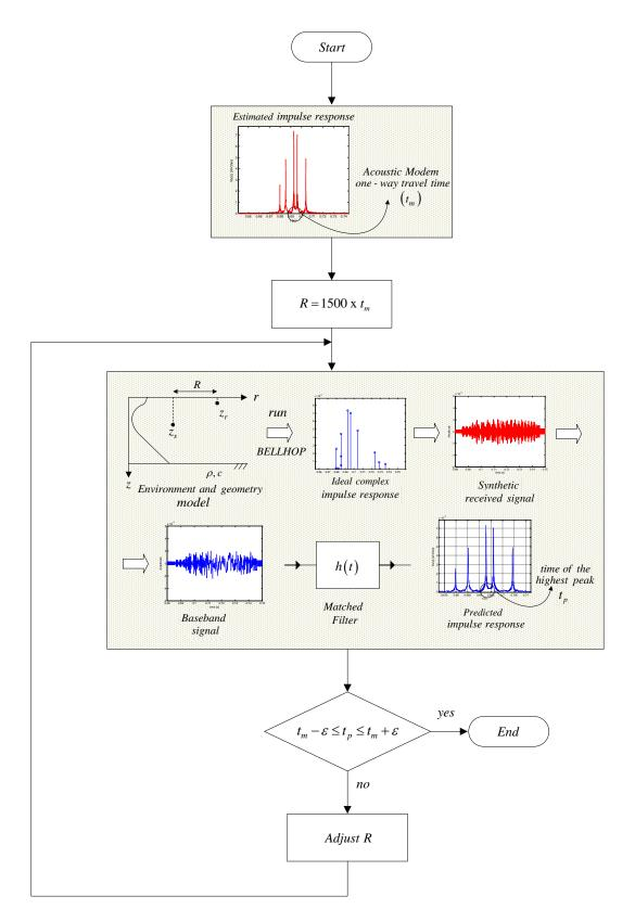
Figure 18. Matched Peak IR Processing Flowchart
