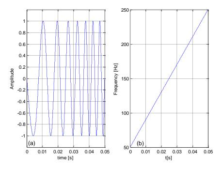
This LFM pulse is defined in the interval 0 < t < 50ms with B = 200Hz (TB = 10).
