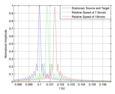
The characteristics of the HFM pulse are: T=50ms, B=5 kHz sweeping from 9 kHz to 14 kHz (TB=250).
